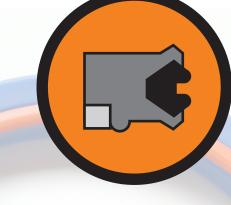
The RP1 U-Cup is recommended in heavy duty demanding hydraulic cylinder application which require high pressure, low temperature and when large extrusion gaps are needed for effective wear ring bearing exposure.
